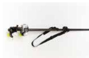
An underwater camera developed by an employee, the camera's arm length can be extended to check a vessel's bottom from onshore. These inspections can be carried out more frequently than diver inspections, so we are able to identify the right time for required bottom cleaning, thus improving fuel efficiency.
